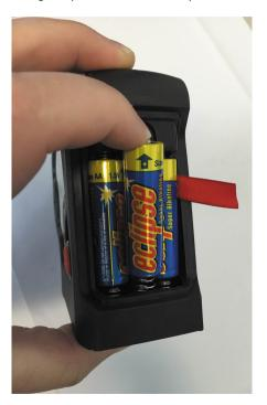
Always use a good quality alkaline battery and never mix new and old batteries for optimum performance and battery longevity.
