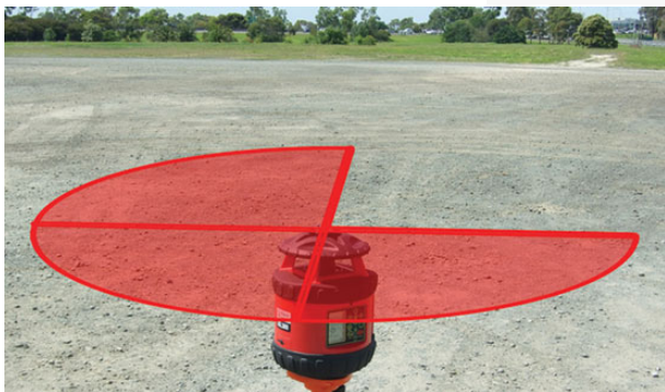
Photo showing one quadrant (90° arc) of rotation with laser output turned off
