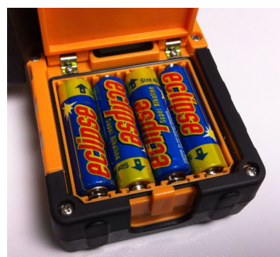
Battery Compartment 4x "AA" Alkaline Batteries
